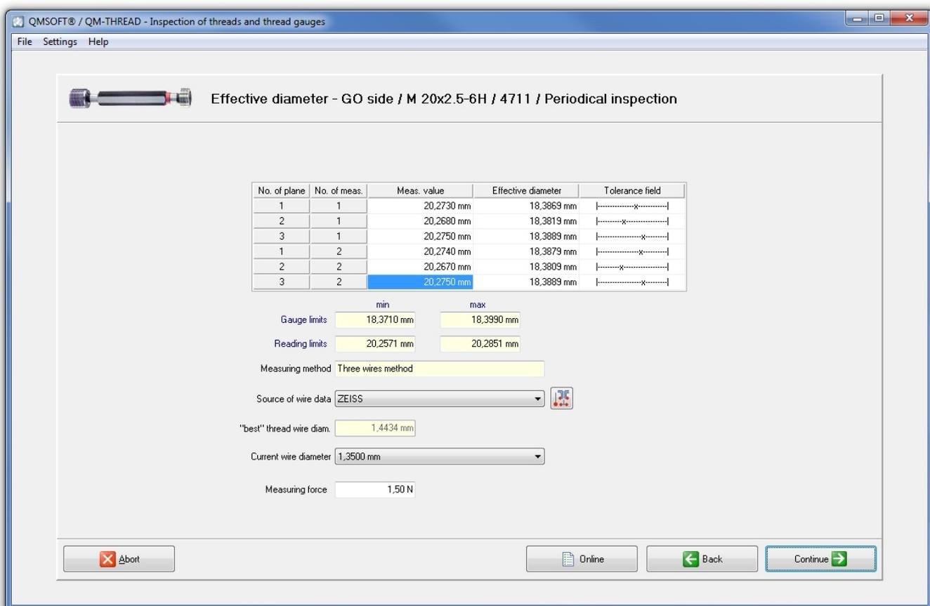
The screenshot displays the QM-THREAD software interface. At the top, it shows the title bar 'QMSOFT® / QM-THREAD - Inspection of threads and thread gauges' and a menu bar with 'File', 'Settings', and 'Help'. Below the menu bar, there is a header area with a small image of a thread gauge and the text 'Effective diameter - GO side / M 20x2.5-6H / 4711 / Periodical inspection'. The main area contains a table with the following data:
