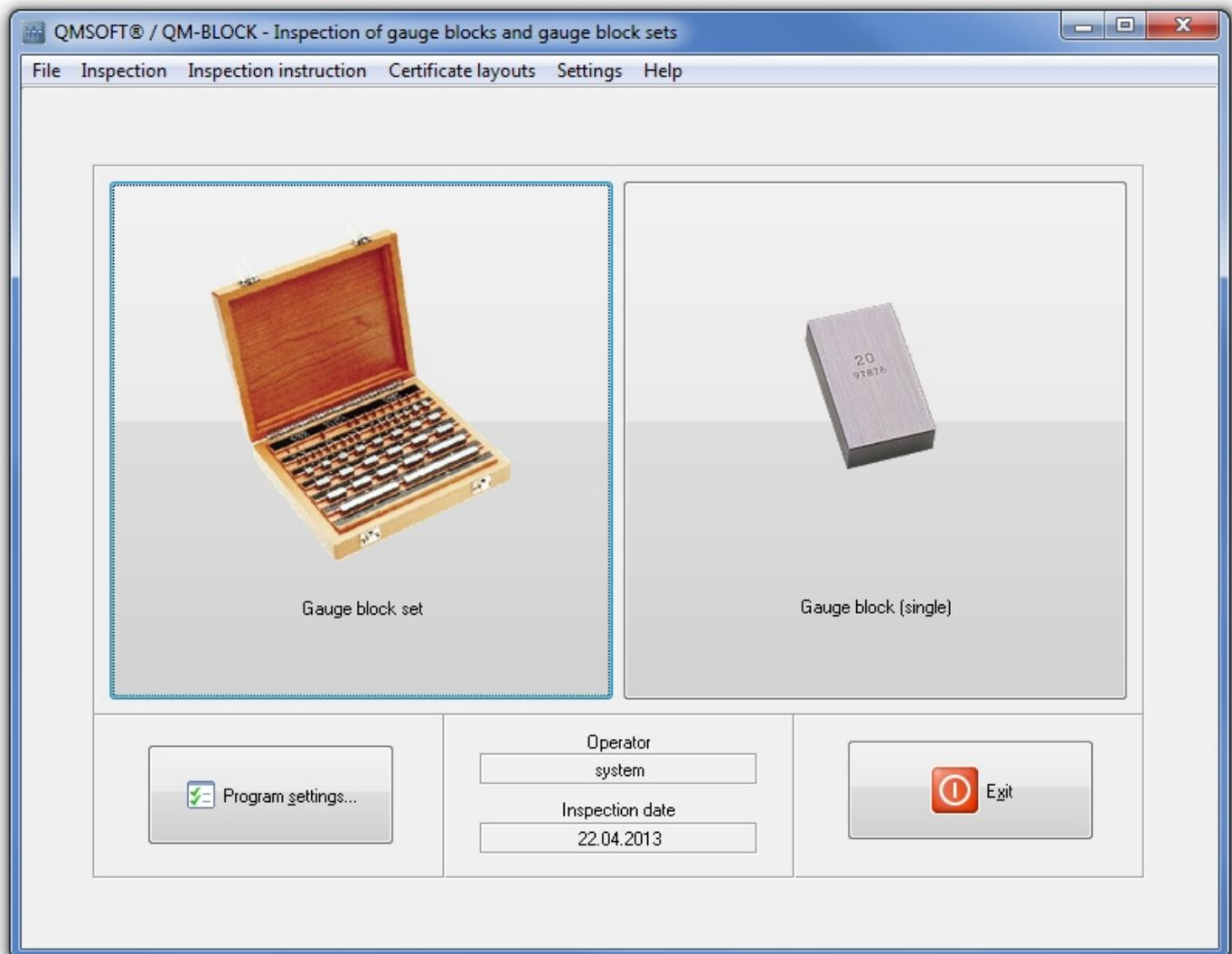
Most gauge block inspections are performed under the application of the method of "difference measurement", i.e. comparing the known actual size of a reference gauge block with the size of the gauge block which is to be inspected.
